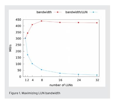
LUNs within a single target share resources (for example, using the same command queue(s) and interrupt(s)), so adding more units will always limit the bandwidth that is available to each LUN.
